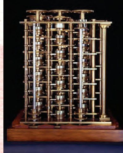
Babbage’s “difference engine,” or automatic mechanical calculator (1822)
