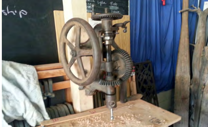
A human-powered post drill used to bore holes in chair legs to accept the rung tenon; this drill was manufactured about 1910.
