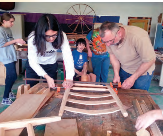
Putting together the back construct by fixing slats and rungs into the two rear legs
