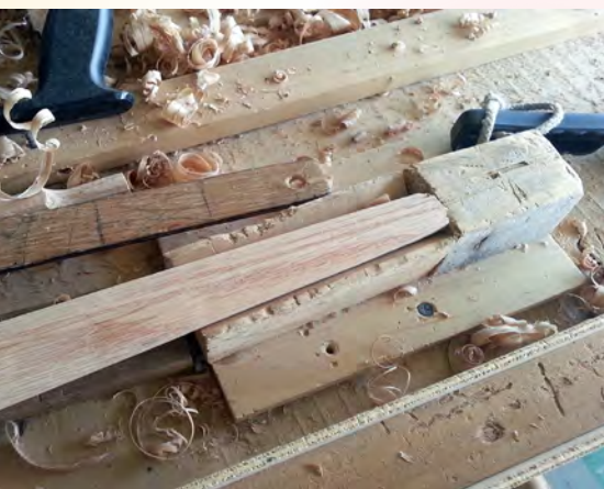
A rear chair leg in a v-block fixture that holds it while it is being shaped into an octagonal cross section
