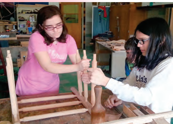
Placing rungs to connect the front and back constructs
