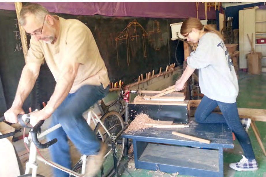
A human-powered lathe cutting the tenon on the end of a chair rung
