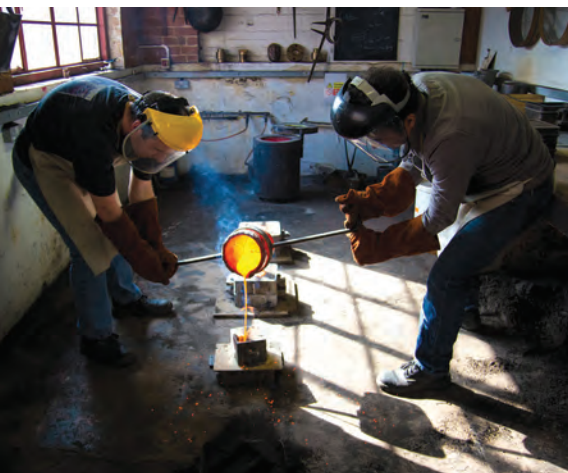
Pouring molten bronze (1800 degrees Fahrenheit) into the mold for a garden trowel
