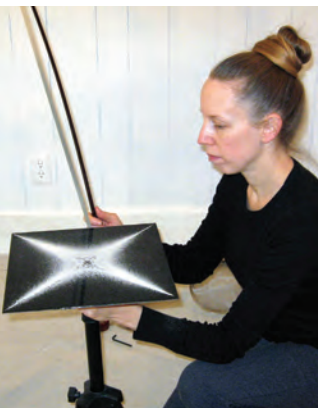
A Chladni plate, covered with fine salt, when stroked by a violin bow will create geometric patterns.
