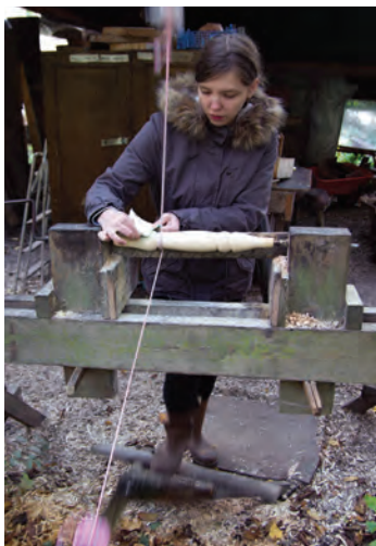
Making a stool spindle-leg on a treadle-driven pole lathe
