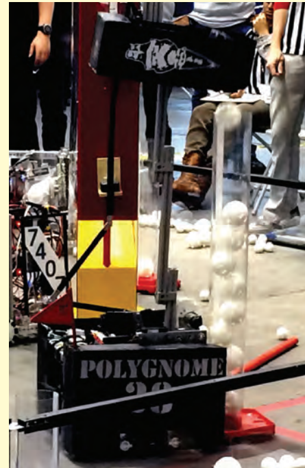
In competition, PolyGnome scoops up wiffle balls off the floor by means of a little spinning paddle and then deposits them in tall plastic tubes.
