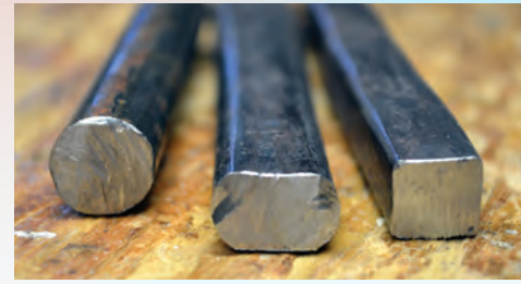
Round stock can be heated and hammered into a bar with a square or a rectangular cross section.
