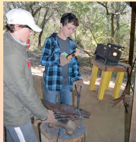
Ninth graders, using hammer and tongs, shape a piece of steel, the propane furnace in the background.
