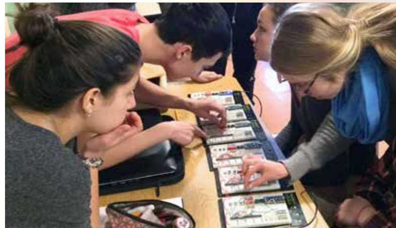
Waldorf tenth graders building a binary addition circuit, i.e., a circuit that can add numbers that are expressed in terms of zeros and ones
