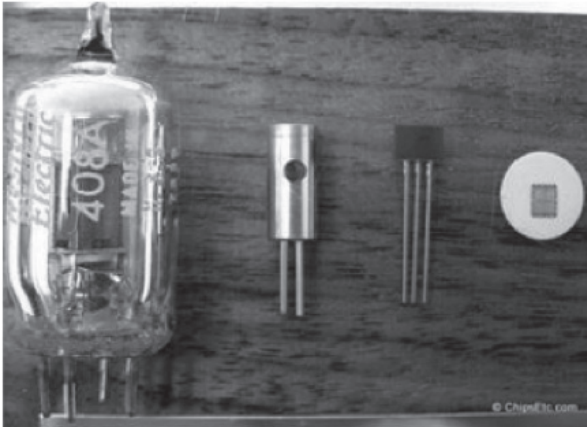
Vacuum tube to transistors to integrated circuits within 25 years (courtesy chipsetc.com)
