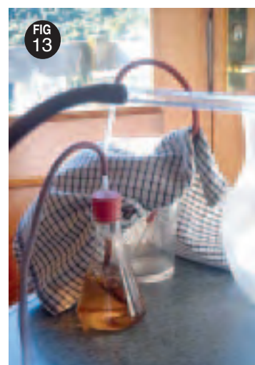
Figure 12: The working kiln with the burner going and a glass tube extending from the calcination tube taking the vented gases through the conical flask containing dilute red cabbage juice.
