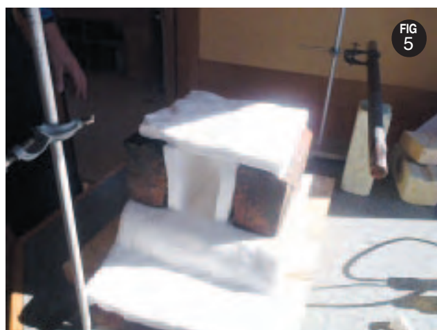
Figure 3: The back of the kiln where the burner will be inserted. Notice the little apron of ceramic fibre wool which forms the base of the fire box and extends out beneath where the burner will be to prevent the heat getting down to the bench.
