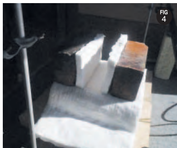
Figure 4: The ceramic fibre lining of the sides of the fire box, which must be just big enough to fit the steel calcination tube with only small gaps around it.
