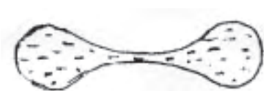
Figure 2 : Cross-section of the squeezed tube in approximately 9 m height, after the water level has fallen to 10 m.
