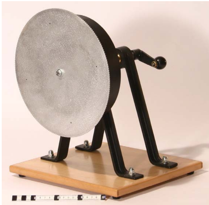
Physics—200 Toothed Disk For Measuring Frequencies
