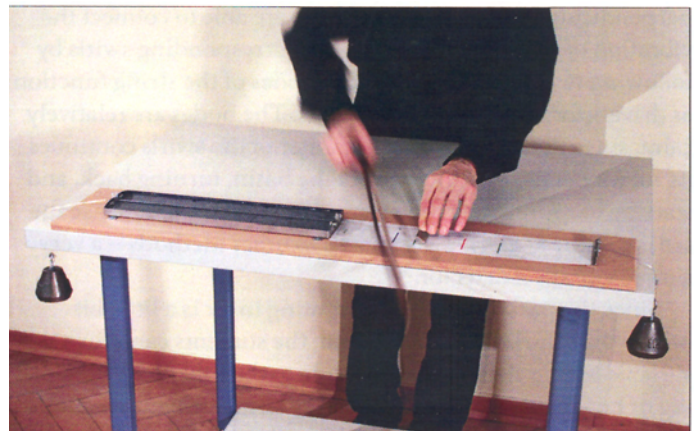
Fig. 1. Hydromonochord being bowed. The string on the left-hand side is just wetted by the water in the basin.
