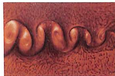
Plate 5. Between laminar flow and turbulence. Spontaneous formation of rhythmically alternating vortices in the wake of steadily moving cylinder (the fluid is a water/glycerine mix, with suspended aluminium dust for visualization). The rhythmic, vortical flow patterns are typical of blood movement through the heart. The central vortex pair in this photograph is similar to the pattern of movements traced by the blood sweeping into the left ventricle.
