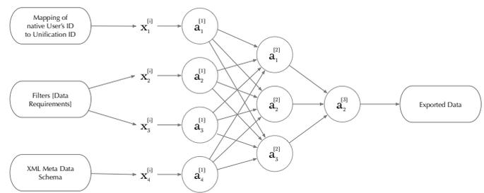
Fig. 6. Phase 3 - Comprehensive Network: Representation commonly used for Neural Networks, where  $x_1, x_2, x_n$  in the first input diagram represent fields from source data. For better aesthetic, the parameters such as weights and biases have been omitted.
