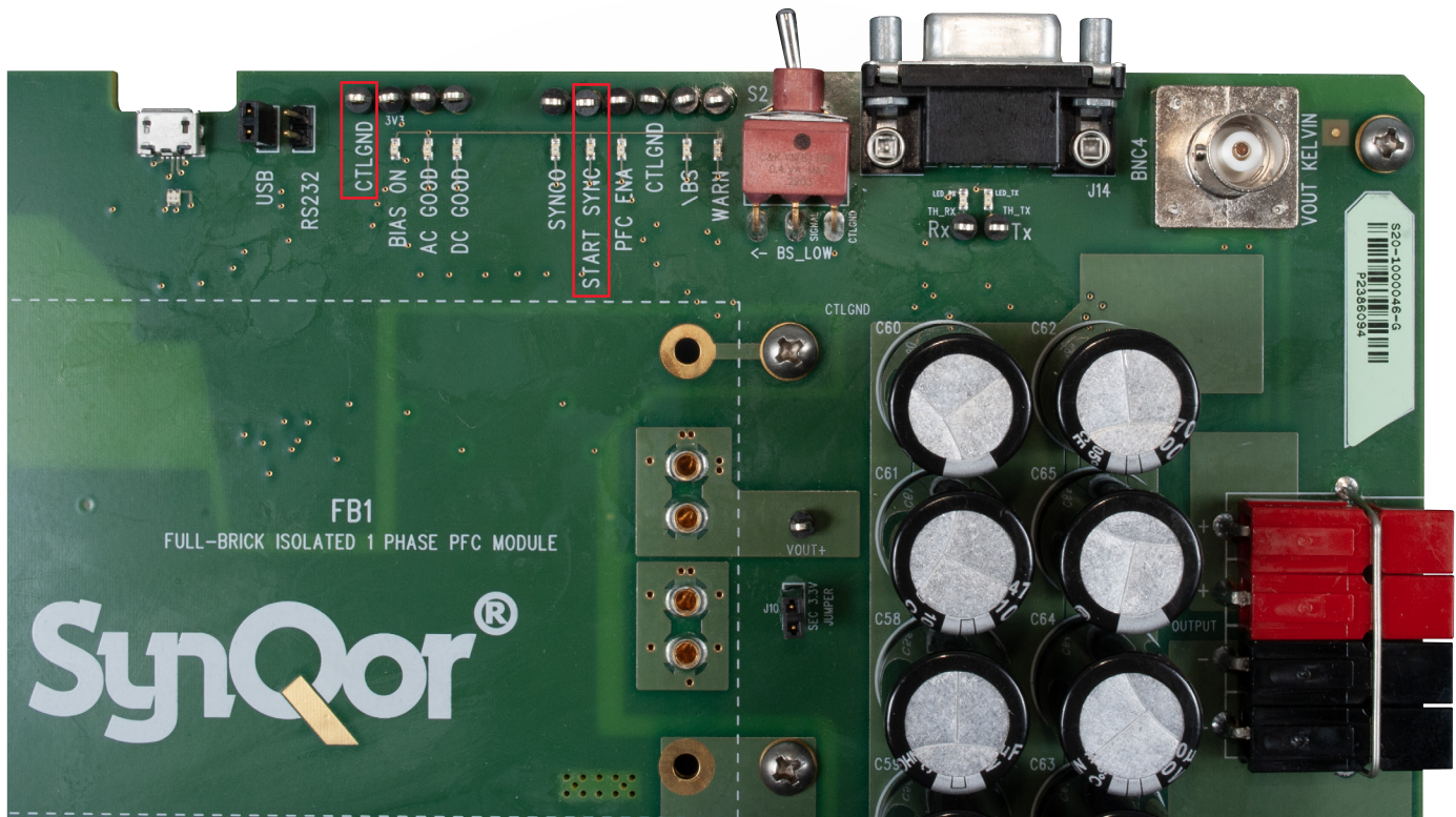
Figure 5: Location of “CTL_RETURN” and “START_SYNC” test points on the evaluation board.
