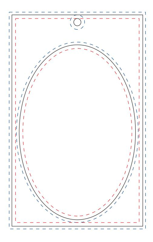
Individual Rectangle Optional Hole Carrier - 4.5"x7.25" / Oval Kiss Cut - 4"x6" / Peg Hole - 0.25"x0.25"
