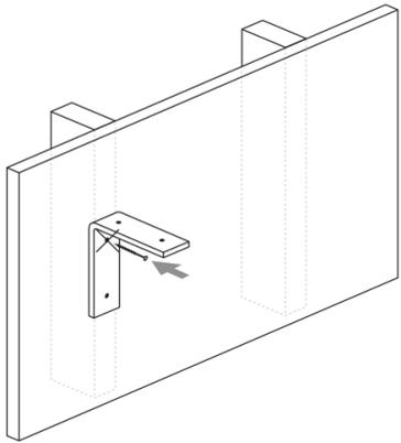
**2** Measure the bracket spacing from screw hole mark, and righteously apply painters tape to general mounting area of second bracket. Measure again and draw a short vertical line on the tape. **See Rad Tip #2 below.**
