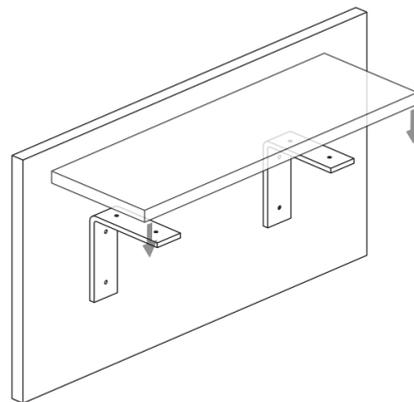
**8** Hold the shelf steady and use a set screw to poke a hole on the shelf. Using your 1/8" drill bit, predrill set screw locations before installing set screws into the shelf.
