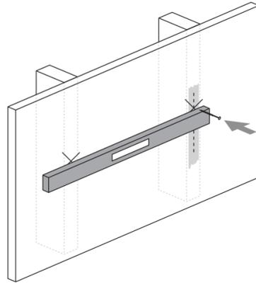
**4** Install the top screw locations. Vertically level each bracket. Punch a hole in all remaining screw locations with screw tip.
