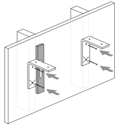
**5** Screw holes that are not on studs or blocking require a wall anchor. Remove the brackets from your wall and predrill applicable screw locations with a 1/4" bit then install wall anchors. Take a swig of your brew.
