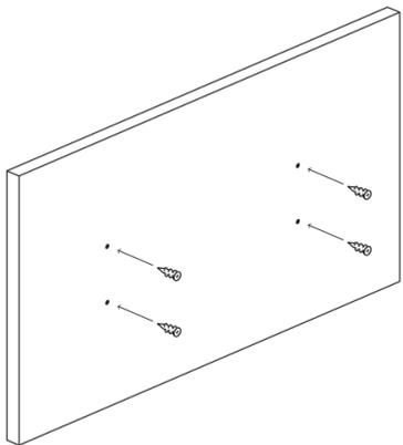
**6** Position the brackets, install all wall screws. Use a level to check each bracket for sag. **See Rad Tip #4 to remove sag.** Confirm the brackets are secure to wall.
