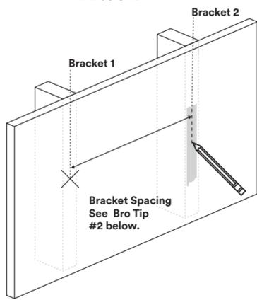
**3** Place a level on first screw hole. Find the intersection at level and vertical line. If you do not have a long enough level, **see Rad Tip #3 below.** Use a wall screw to punch a hole into the wall behind painters tape. Remove the tape.
