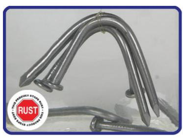
Test performed with distilled water & Zerust® Capsule<sup>™</sup> submerged 48 hours prior to adding metal.
