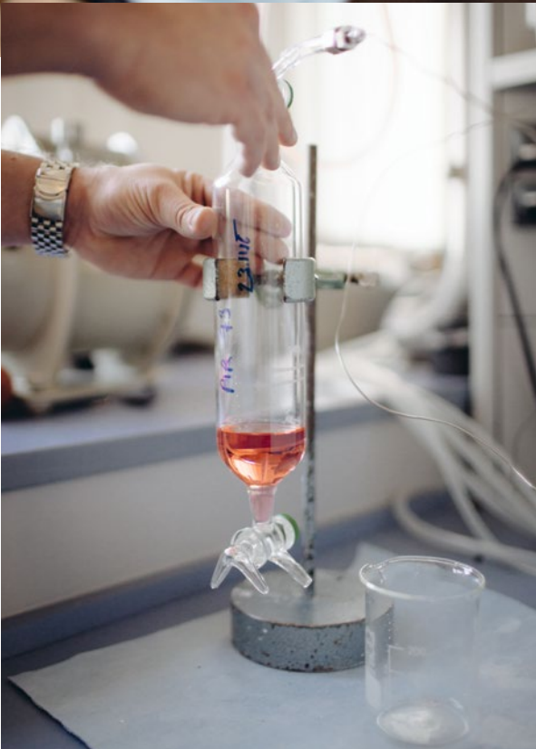
For gas sample collection in the field, the TECH Center & Lab team uses special glass cylinders.
