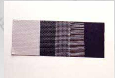
**Sarnafil's Reinforcement Becomes Embedded in Polymer During a Coating Process**
