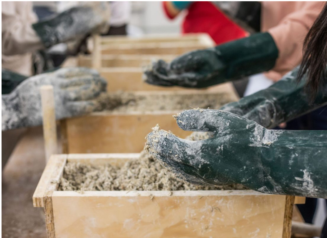
Fig 1.4 Filling molds with Hemp and Lime mixture for pre-cast components
