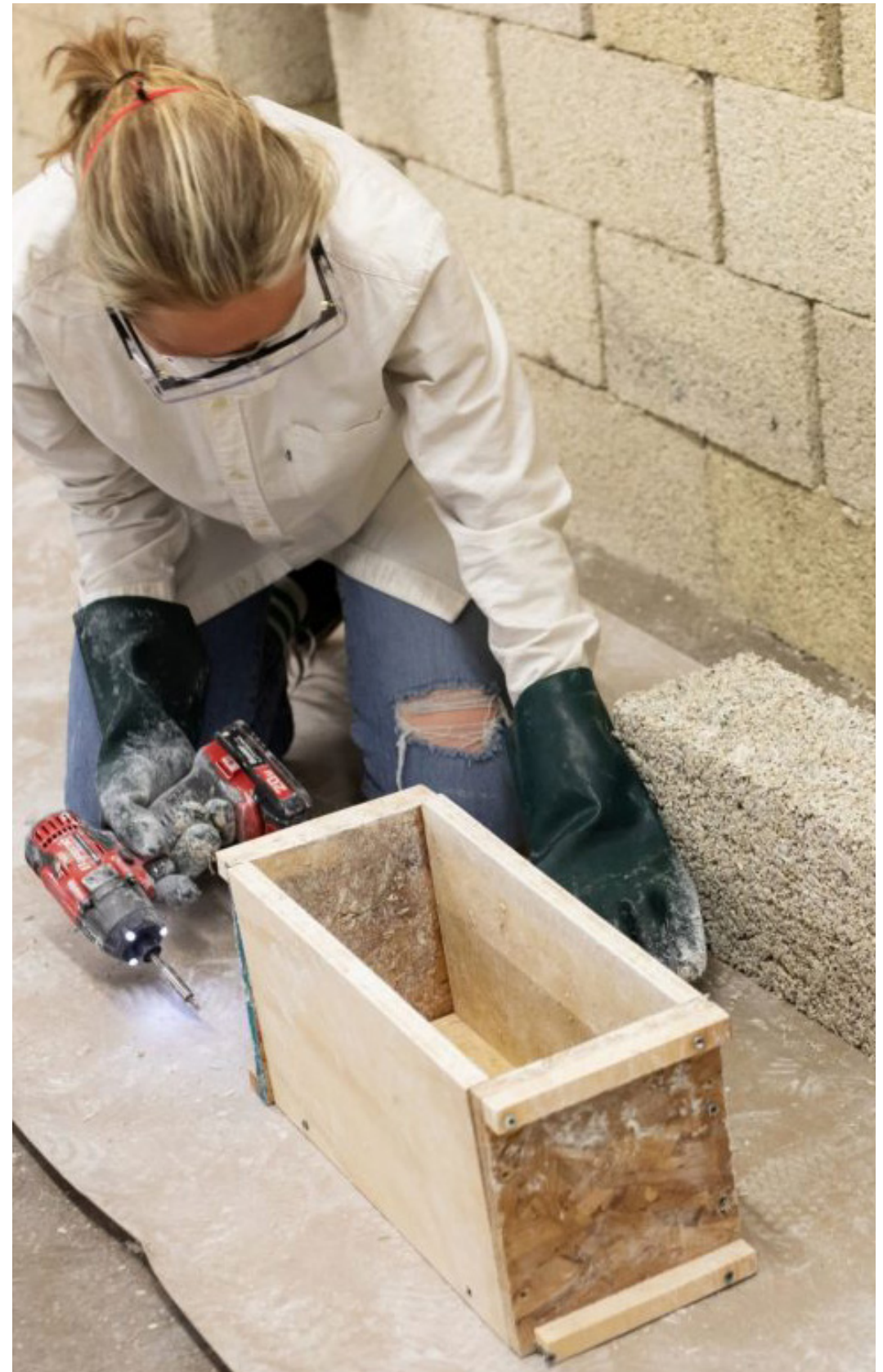
Fig 1.1 Wood mold assembly
