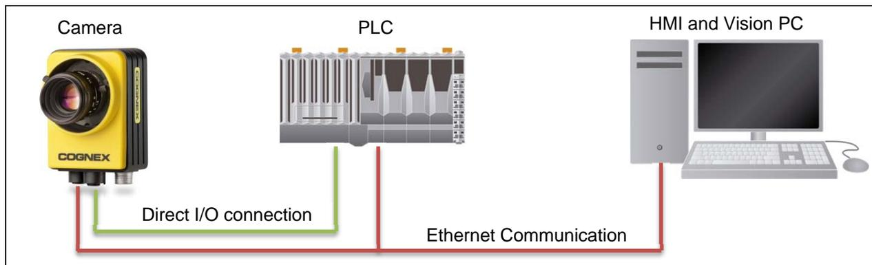
Figure 1: Traditional Vision to PLC system
