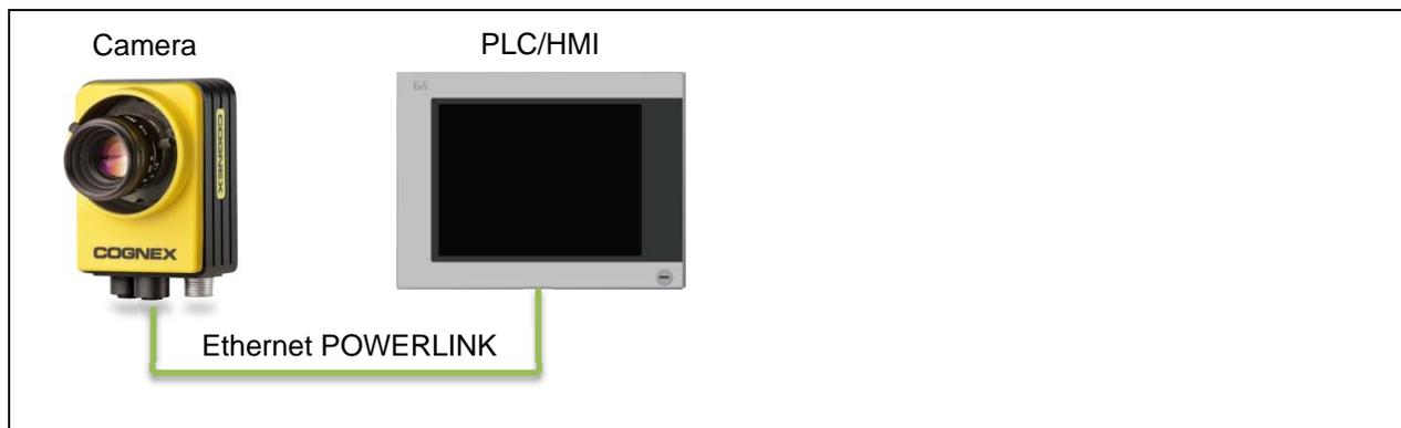
Figure 2: Modern Vision to PLC system
