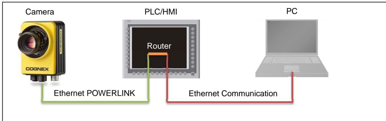
Figure 4: Using the PLC system as gateway
