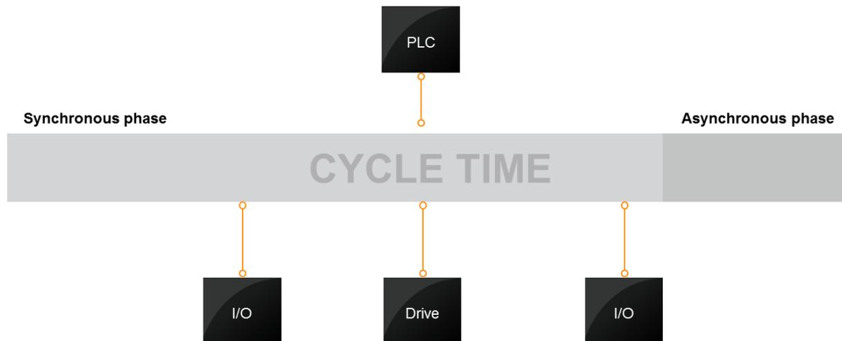
Figure 3: Real-time Ethernet cycle
