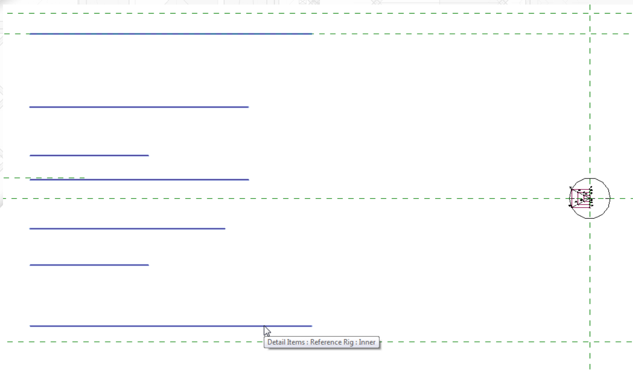
FIGURE 12—INSERT THE REFERENCE RIG TO CONTROL THE RADII OF THE INNER FILLET ARCS
