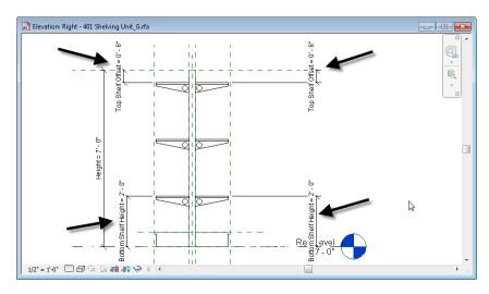
Using formulas, we can set the quantity of shelves in a few ways. One very common approach is to create a conditional statement that prevents the Array from failing if someone inputs a bad value. In the case of a linear array, we need at least two items, so a bad value is less than 2. To create such a formula, open Family Types, and create a new parameter of the type: **Integer**. In the formula column input:
