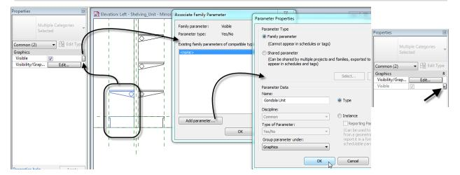
A small equals (=) sign will appear on the button to indicate that it is now driven by a parameter.
