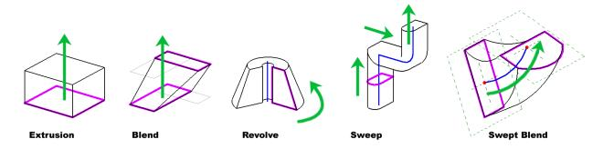
An extrusion is a sketched shape pushed along a distance perpendicular to the sketch plane. A blend is similar accept that instead of a single shape, you have both a top and a bottom shape
