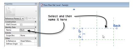
6. Add dimensions (Modify tab or type DI) to each group of Reference Planes. Two vertical and two horizontal. There should be an overall and a continuous string including the centerline in each direction.
