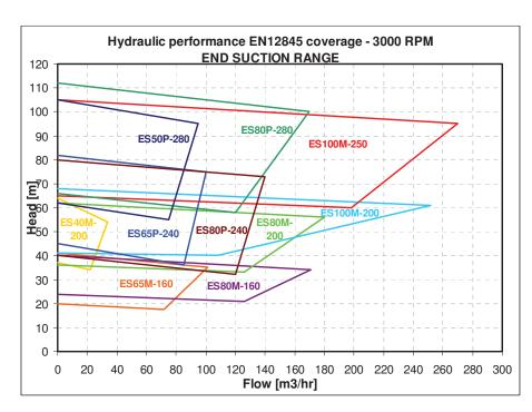
Based on a maximum pump NPSH required of 5m, the Patterson End Suction product line performance ranges up to 270m<sup>3</sup>/hr, and up to 105m head.
