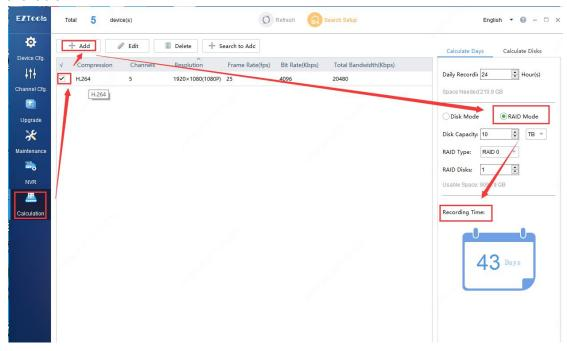
Calculate how many RAID disks are needed based on the daily recording period (hours), recording retention period (days), RAID disk capacity available, and configured RAID type.
