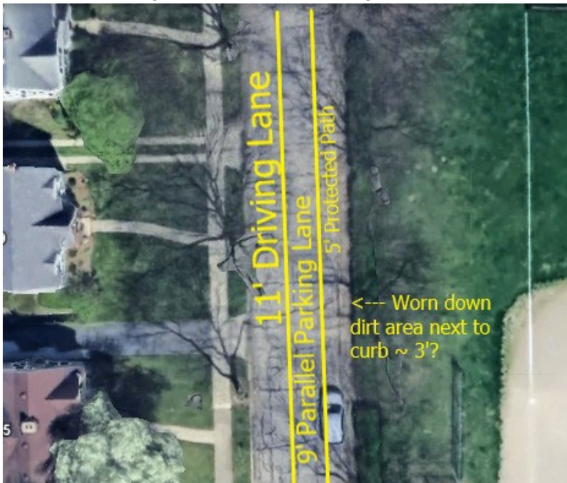
Image 2: Curve at Osborn and where markings are needed to (1) stop incoming traffic, (2) indicate no parking/stopping areas. (Potentially angle parking on North and add angled parking on South to provide further visual cues that section is one way)
