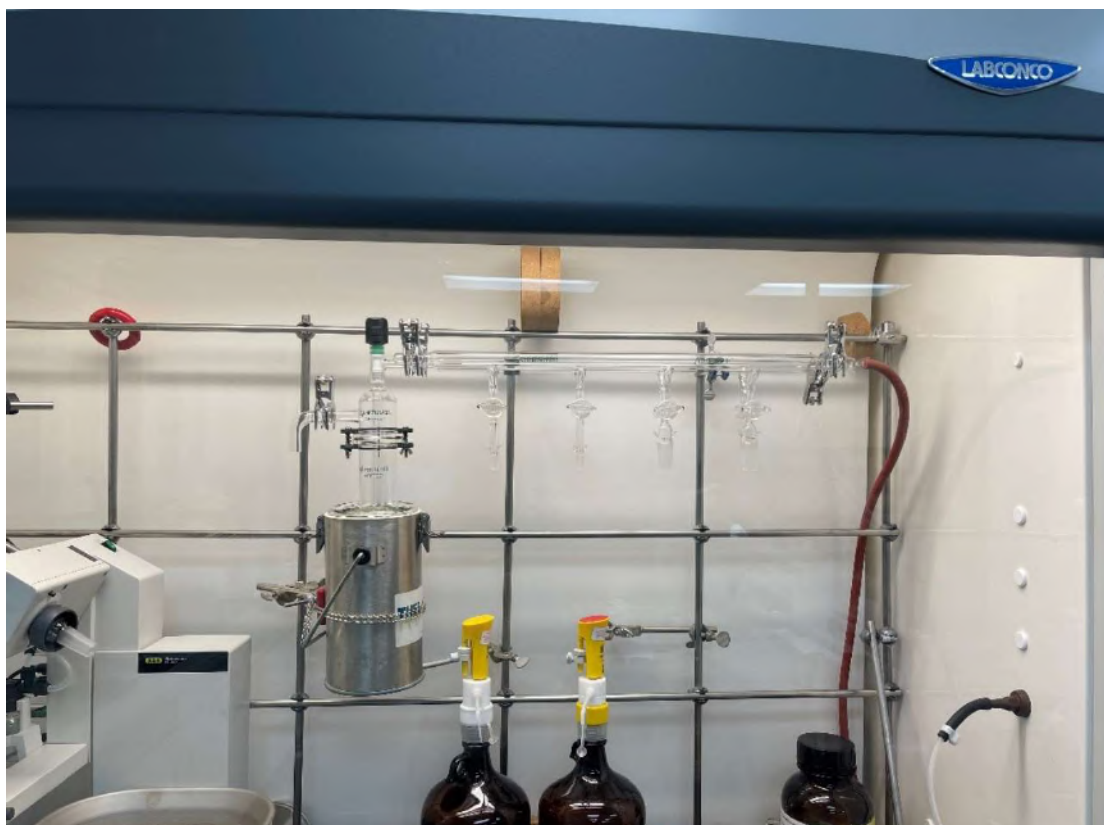
Above: Schleck Line for synthesis requiring inert nitrogen or argon atmosphere.
