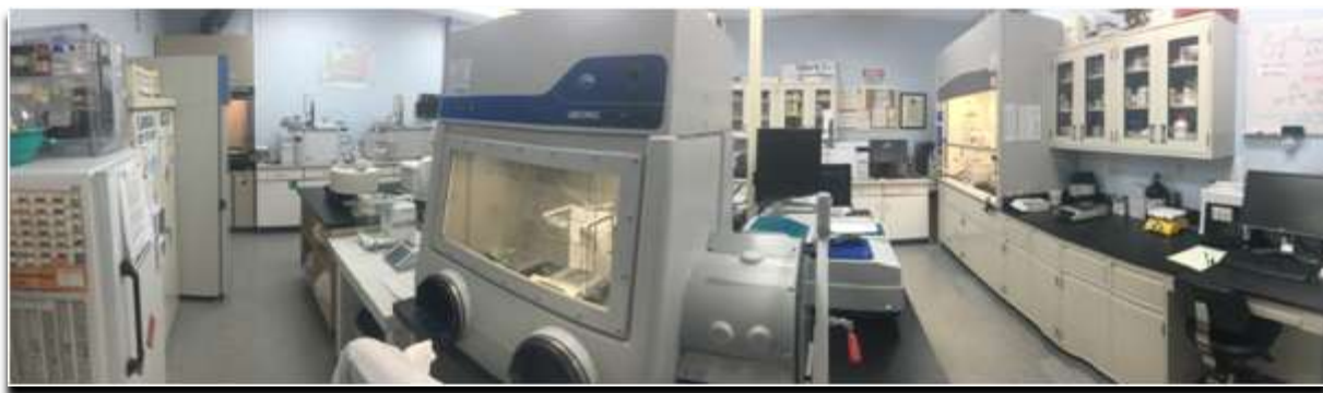
Above: Labconco, Inc. Dual HEPA-filtered Glovebox with a Semi-Micro Analytical Scale for weighing highly poisonous/unknown compounds.
