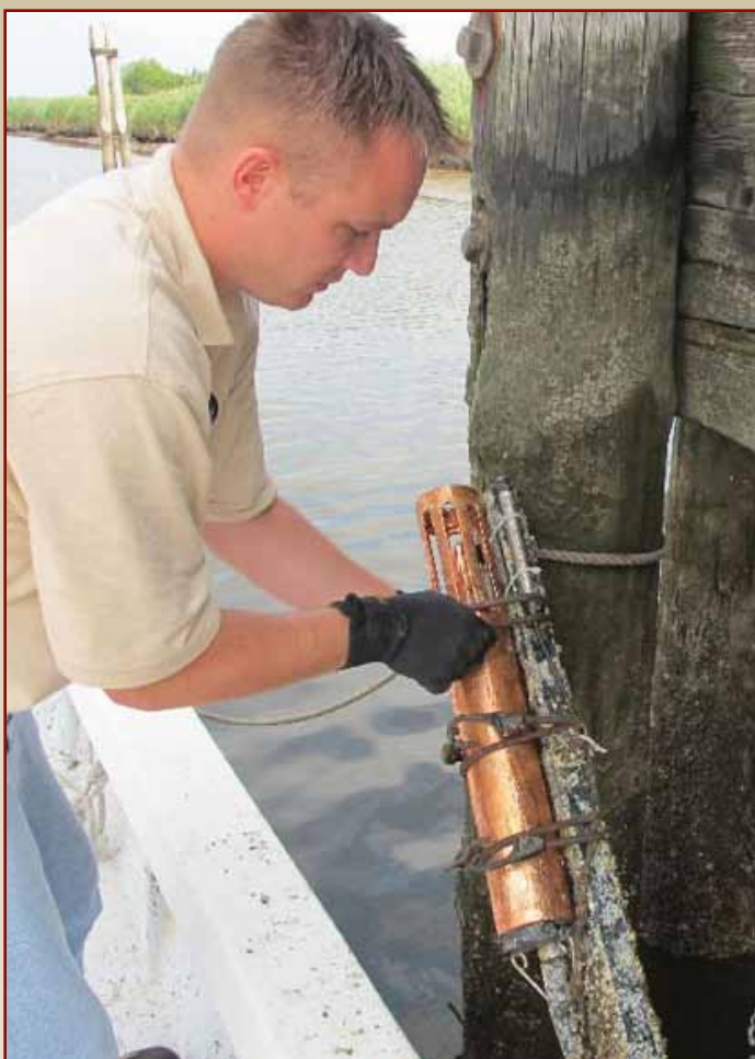
MERI staff performs maintenance on water quality sensor
