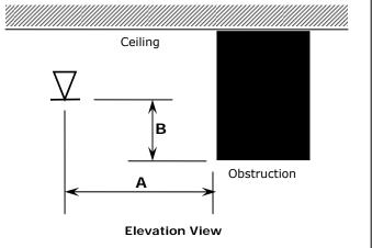
From: NFPA 13D, FIGURE 8.2.5.4.2, Position of Sprinkler to Avoid Obstructions to Discharge
