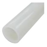
Uponor AquaPEX white tubing is marked with the PEX 5106 designation as required by the most recent edition of ASTM F876-15a, indicating it exceeds ASTM F876 chlorine-resistance requirements for continuous-recirculation systems operating up to 140°F while also affording a one-month UV-resistance level. Uponor AquaPEX white tubing ( ¾", 1" and 1¼" only) is also listed to UL 1821 and ULC/ORD-C199P and carries an additional rating of 120°F at 130psi.
