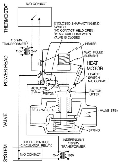
the boiler control (T T) and separate system transformer. The relay in the boiler (or zone control box) starts the circulator. The piston continues to move down until the valve is fully open.
