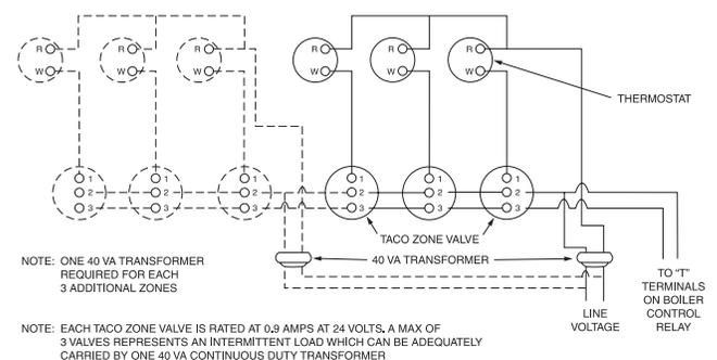
Figure C: Zone Valve Circuits.
