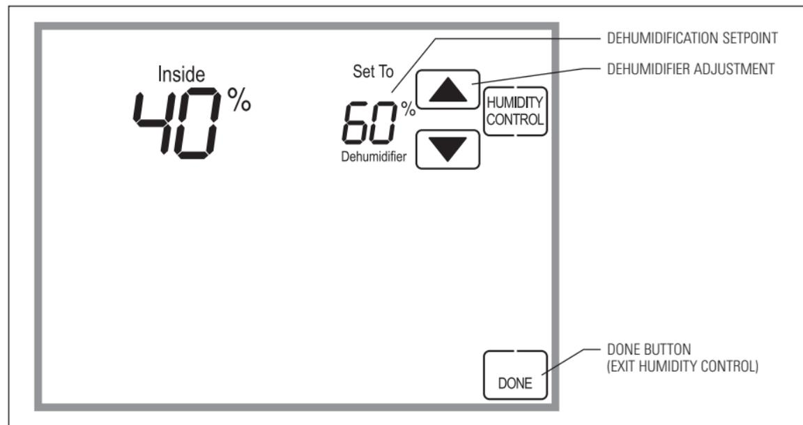
If dehumidification is done with the air conditioner, the Home Comfort Control will cool up to 3°F beyond the cooling setpoint for dehumidification. Note overcooling may not be sufficient to meet the dehumidification setpoint.
