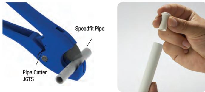
To prevent damage to the O-ring remove all burrs and sharp edges. When using Speedfit® or other types of PEX Pipe, we recommend the use of Pipe Insert.
