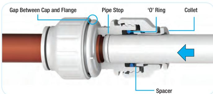
The fitting should be in the 'unlocked' position. This is shown by a small gap between the screw-cap and the body flange.
