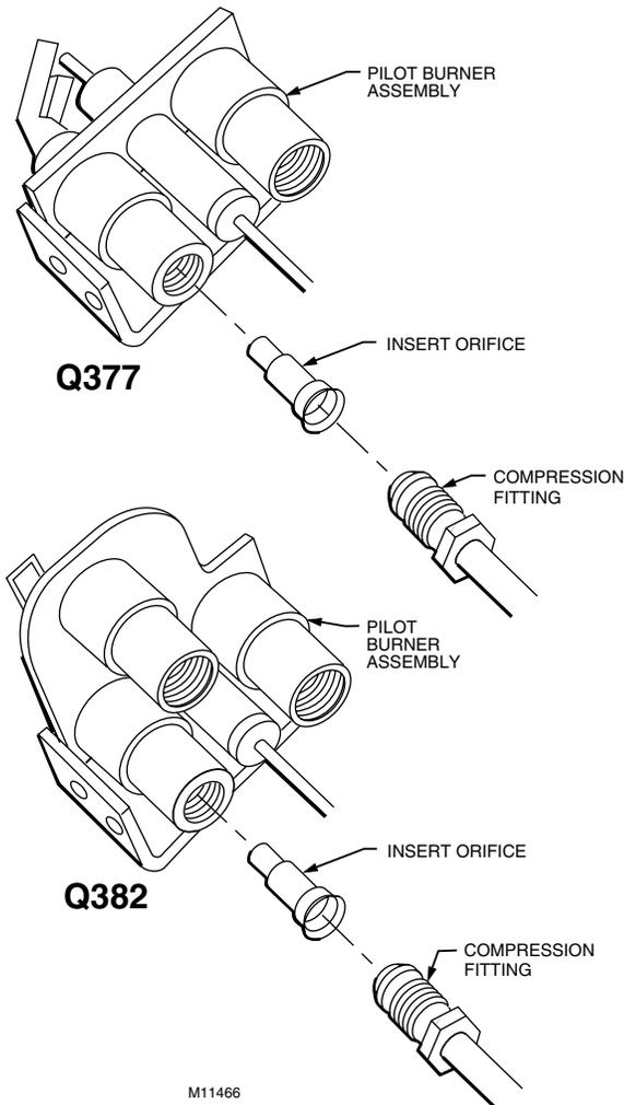
Fig. 23. Changing insert orifices (Q377 and Q382 shown).
