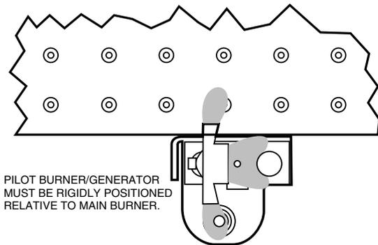
PILOT BURNER/GENERATOR MUST BE RIGIDLY POSITIONED RELATIVE TO MAIN BURNER.
