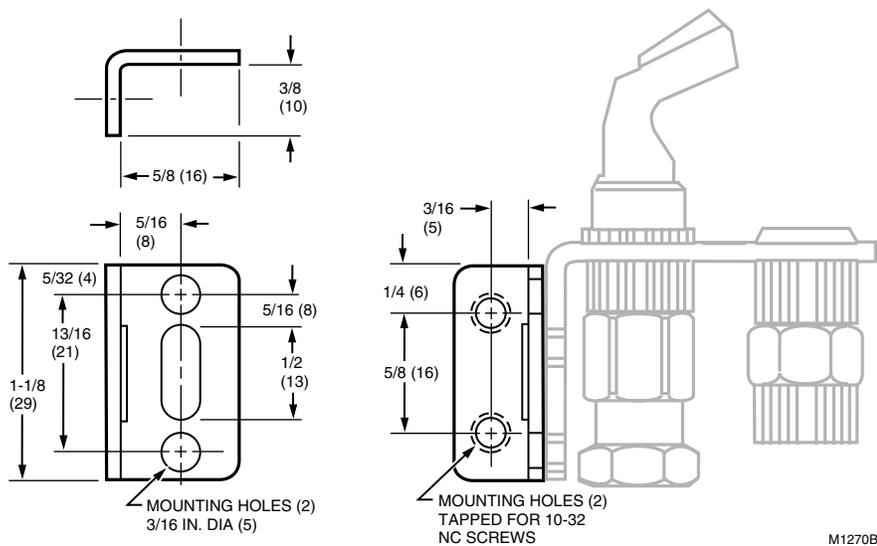
Fig. 16. Tradeline Q314 "A" mounting bracket adapter dimensions.
