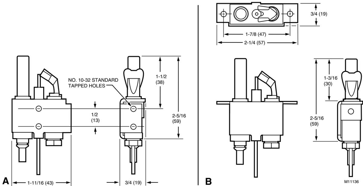
Fig. 13. Q379 mounting brackets and dimensions in in. (mm).
