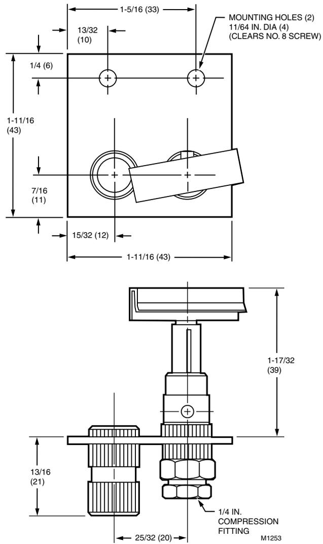
Fig. 14. Q380 No. 1 mounting bracket and dimensions.
