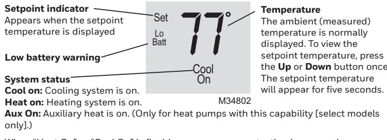
When "Heat On" or "Cool On" is flashing, compressor protection is engaged.
