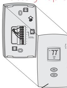
Pull at bottom to remove thermostat from wallplate.
