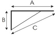
ACB-30: (A)30" (B)16" (C)34" ACB-36: (A)36" (B)16" (C)39" ACB-42: (A)42" (B)16" (C)43" ACB-48: (A)48" (B)16" (C)51"
