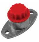
rendering it leak proof. It withstands continuous operating temperatures of  $165^{\circ}F$  ( $72^{\circ}C$ ) and intermittent spikes up to  $215^{\circ}F$  ( $100^{\circ}C$ ). Port cap has exceptional dimensional stability and is impervious to most chemicals and freezing temperatures down to  $-94^{\circ}F$  ( $-70^{\circ}C$ ).
