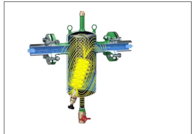
For the steel DIRTMAG®, the ferrous impurities are captured by a concentrated magnetic field created by a stack of neodymium rare-earth magnets positioned inside a brass dry-well below the flow stream.
