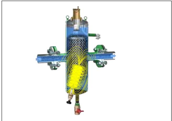
For the steel DISCALDIRTMAG®, the ferrous impurities are captured by a concentrated magnetic field created by a stack of neodymium rare-earth magnets positioned inside a brass dry-well below the flow stream.
