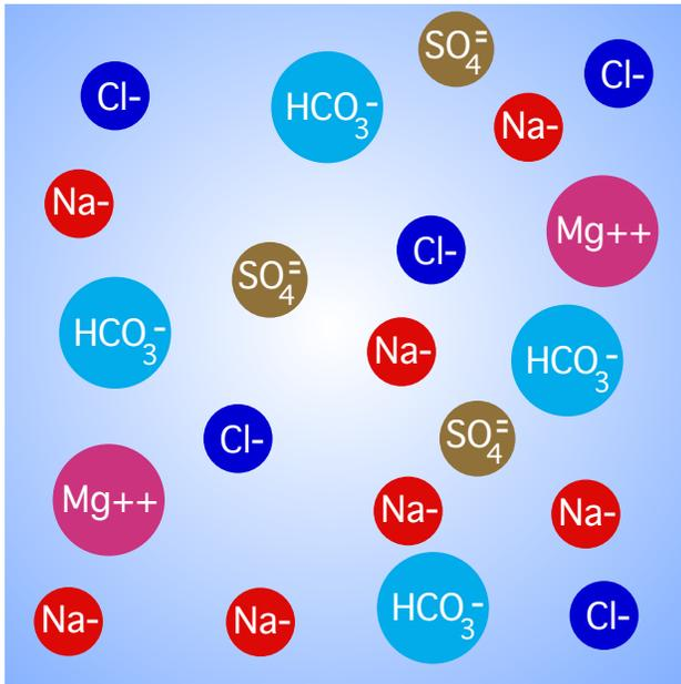
The higher the temperature of the surface in contact with the water, the greater the potential for scale formation. This is why scale often forms on the bottom of tea kettles.
