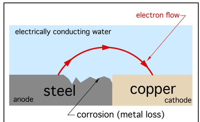
The loss of electrons from the steel will eventually show as pitting and the characteristic orange color of oxidized iron.
