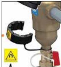
To purge the ferrous impurities in the steel DIRTMAG®, the flexible magnetic stack is removed from the brass dry-well and, with the system still running, the drain valve is opened. Aided by the system pressure, the dirt and ferrous impurities, including magnetite, flushes out quickly and effectively.
