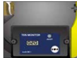
Highly accurate built-in TDS meter 0 - 999 ppm with resolution of 1 ppm due to its advanced microprocessor technology. Auto-Off function conserves battery power. The unit shuts off automatically after 10 minutes of non-use. Replaceable battery with a life of approximately 1000 hours of continuous use.
