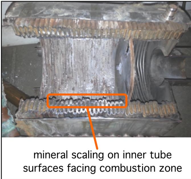
The estimated increase in fuel use due to scale formation, based on research at the University of Illinois and U.S. Bureau of Standards, is shown in figure 2-6.
