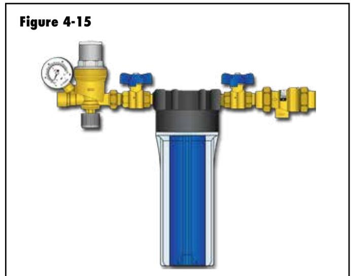
This assembly uses a special 10-inch cartridge insert containing the color changing resin beads necessary to demineralize water passing through it at relatively low flow rates. The cartridge assembly can be isolated by closing the two ball valves. The clear housing can then be unscrewed to remove and replace the cartridge.
