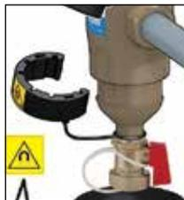
To purge the ferrous impurities in the steel DISCALDIRTMAG®, the flexible magnetic stack is removed from the brass dry-well and, with the system still running, the drain valve is opened. Aided by the system pressure, the dirt and ferrous impurities, including magnetite, flushes out quickly and effectively.
