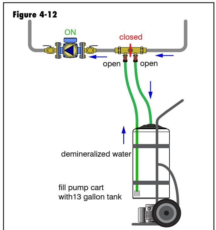
If the system has many branches that require individual purging, and thus, prolong the time over which purging is required, it is possible to fill a *clean* pump cart tank with demineralized water from the HYDROFILL, and then continue the purging process using the cart pump to circulate demineralized water through the system until all air is purged. This is shown in figure 4-12.
