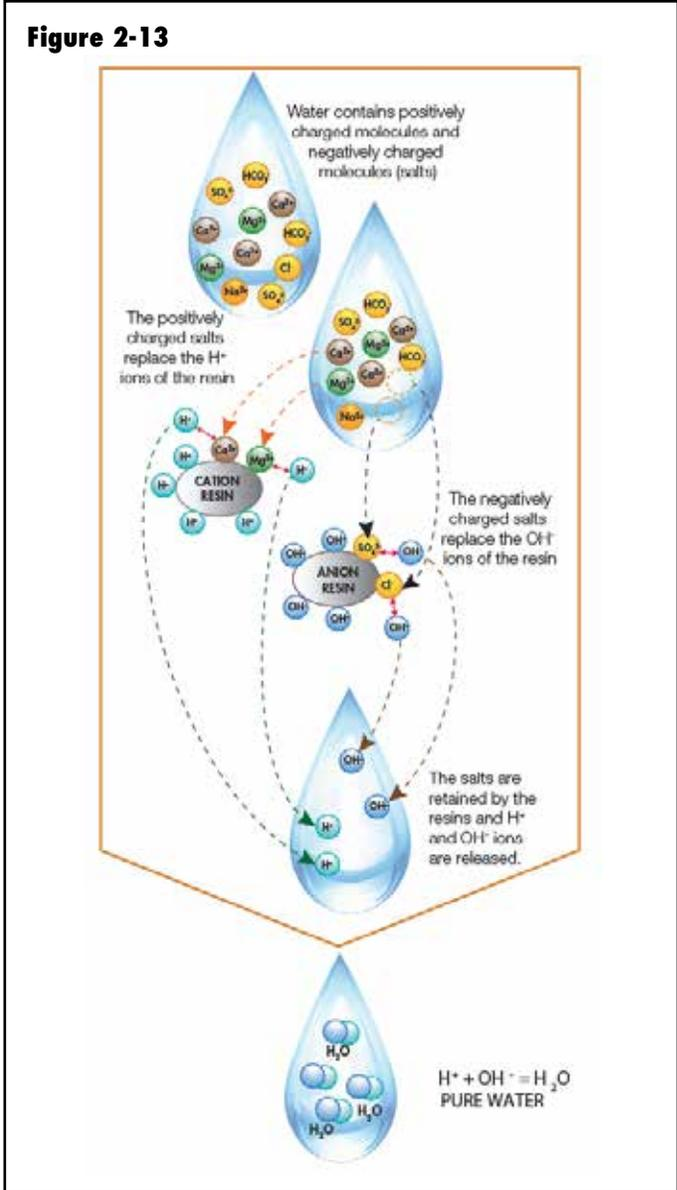
exchange also occurs when a single magnesium cation ( $Mg^{++}$ ) enters a resin bead and is exchanged for two ( $H^+$ ) cations. A sodium cation ( $Na^+$ ) being captured within a bead only releases one ( $H^+$ ) cation. In all cases, the total positive charges of the cations captured equal the total positive charges of the hydrogen cations released from the bead. Thus, the bead remains electrically neutral.
