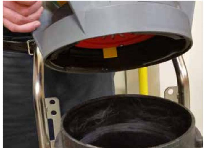
The body is designed to hold highly permeable bags containing the resin beads needed to demineralize water. These bags are simply lowered into the top of the body, as shown in figure 3-4.
