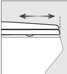
**Adjust seat front to back for proper fit.**
