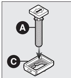
Insert (A) with arrow as shown into (C).
