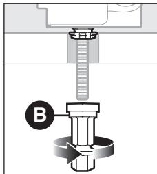
Finger tighten (B) to the under side of the bowl.
