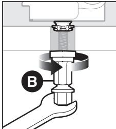
**Holding seat centered on bowl, tighten (B) until lower portions snap off.**
