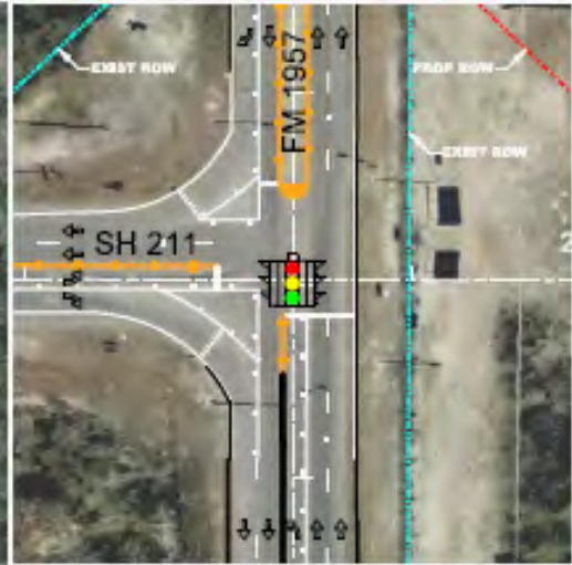
EXISTING SH 211 / FM 1957 INTERSECTION DETAIL AFTER FM 1957 EXPANSION PROJECT CSJ: 2104-02-027
