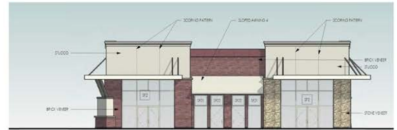
2 EAST ELEVATION - BLDG 1 SCALE: 1/8" = 1'-0"
