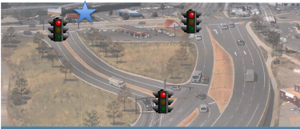
The 8th Street quadrant intersection provides significant capacity and operational improvements to the entire I-25 and Cimarron Street (US 24) interchange facility
