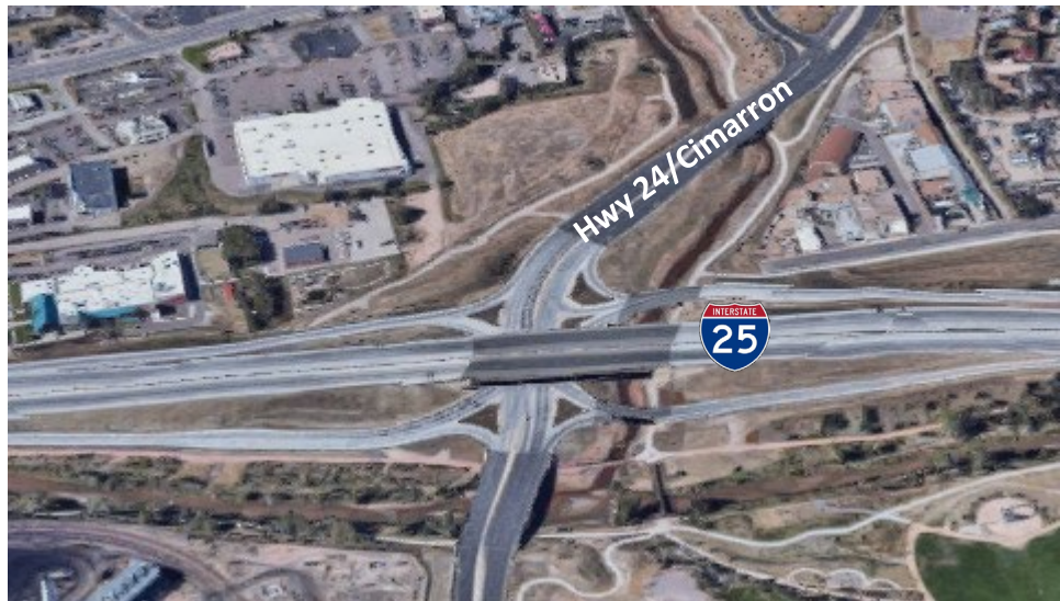
The 8th Street quadrant intersection provides significant capacity and operational improvements to the entire I-25 and Cimarron Street (US 24) interchange facility
