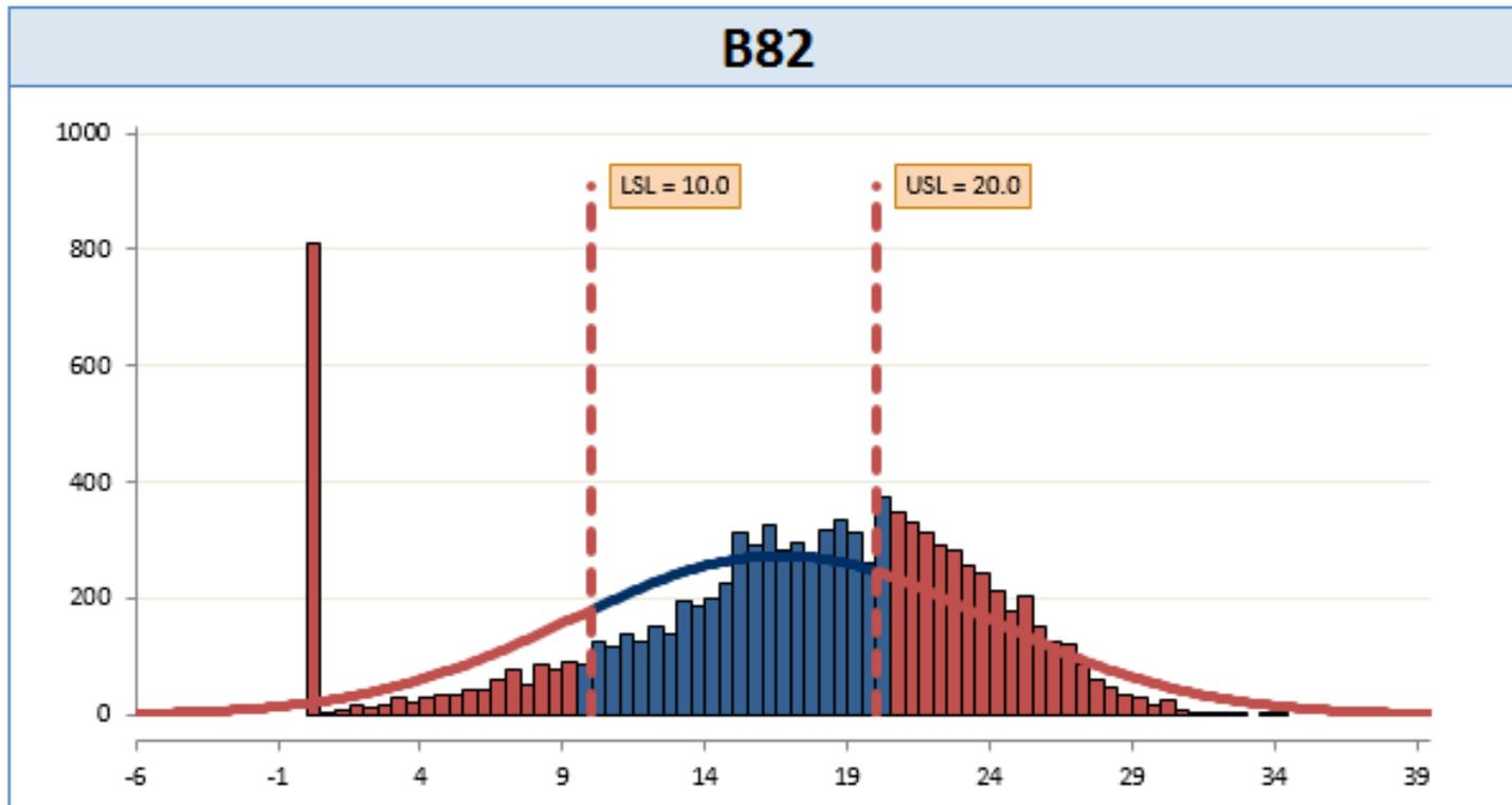
This is the probability distribution of “tilt” measurements for a 15 deg flight with random combination of possible systemic errors.
