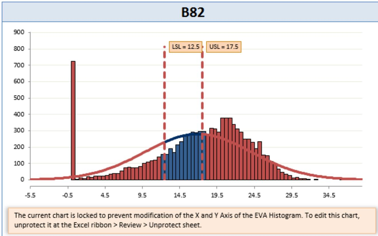
This is the probability distribution of “tilt” measurements for a 15 deg flight with random combination of possible systemic errors.
