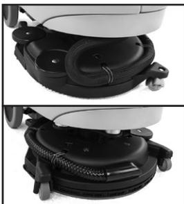
The SC351's rotating deck allows for both forward and backward scrubbing. Operators can push the machine forward in all directions like a "normal" scrubber. But, if the application requires, operators can quickly flip the machine up, triggering the deck to rotate completely for backward scrubbing performance. The scrub deck efficiently guides the wheels for superior edge cleaning.
