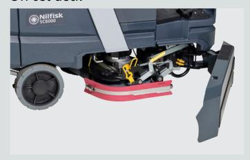
The enclosed off-set deck provides high quality edge cleaning without any added complexity or cost.
