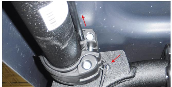
9. Route ROPS Harness along inside top side ROP to front A pillar and secure with (2) Zip Ties.
