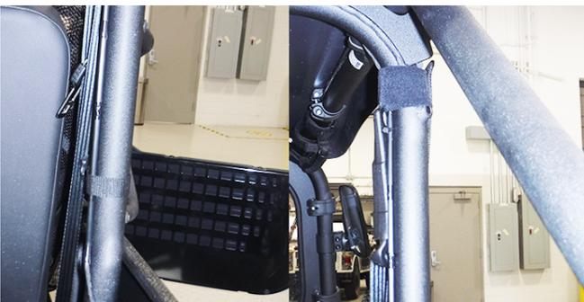
8. Attach second Ribbed Push Clip to top front B pillar into position shown.
