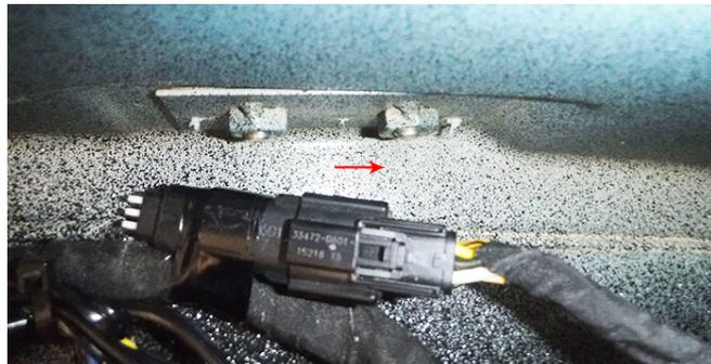
2. Plug connector for ROPS Harness into this plug under passenger side Dash Panel.
