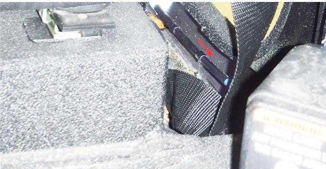
6. Route ROPS Harness to front bottom of B pillar behind seat belt and attach first Ribbed Push clip.
