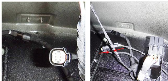
3. Route ROPS Harness along passenger side of vehicle, attaching (5) Medal Panel Clips to edge.
