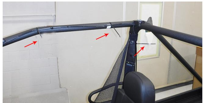
10. Use (2) zip ties to secure ROPS Harness to B pillar top and bottom. Trim excess from zip ties.
