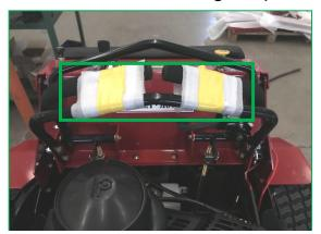
9.Put the four vertical posts in front of the front tire and then lift the mower up to the highest cutting position, push the mower until the back mower fully contact with the crate
