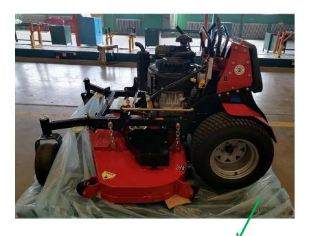
When driving the mower off, notice the base of the crate to avoid trip over
