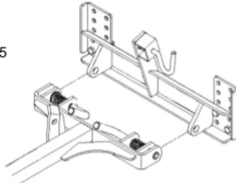
6. After installing the forward arm hitch, adjust the hitch up or down on the bracket to make the platform as level as possible. (Figure 6)
