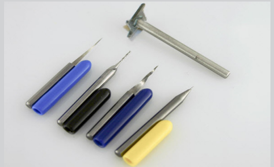
(L - R) 6-degree tapered, 0.032" Flat, 10-dgr tapered, 0.016" Flat, 12-mm hollowing.
