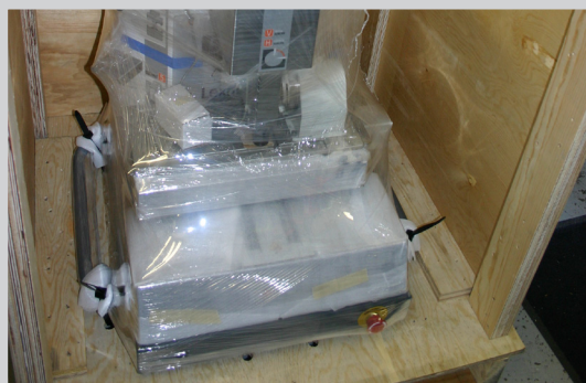
3 - Remove front and back of crate BEFORE removing sides. Set aside screws for when you need to re-use the crate.
