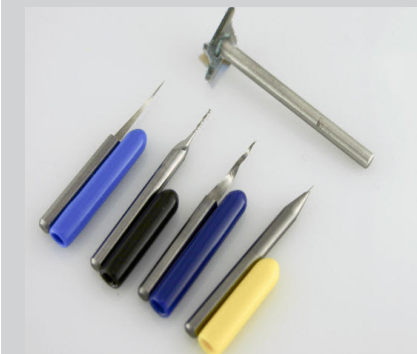
L - R: 6-dgr tapered, 0.032" straight, 10-dgr tapered, 0.016" straight, 12 mm hollow.
