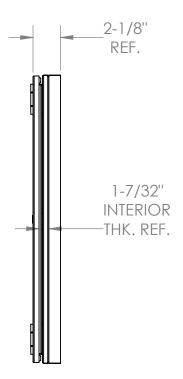
Walnut framing shall be stained first and then clear-coated. Oak framing shall be clear-coated only. Door shall be 1/8" acrylic. Door to be equippped with nickel hinges and built-in lock with keys. The back panel of the case shall be fitted with optional vinyl, cork, tackboard, Porcelain, or changeable letterpanels for interior use. Available Sizes:
