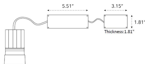
2-sectional driver and wiring box will ship when the AT/CP option is selected. Also can be used for plenum space issues.
